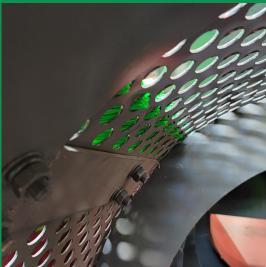
Screening materials: earth, sand, gravel, compost, wood chips, construction waste, recycling material, slag, crushed stone and stone in grain sizes from 2 mm to 80 mm
